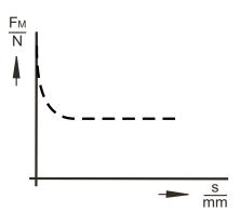
Fig. 2: force vs. stroke characteristic within the nominal stroke
