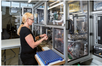
Fully automated assembly and leakage test of tubes
