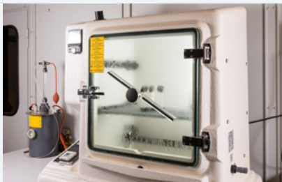
Kesternich chamber for corrosion tests
