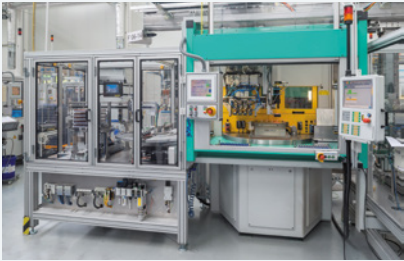
Fully automated plastic encapsulation of solenoid bodies
