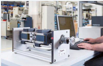
Remagraph for measuring of magnetic properties
