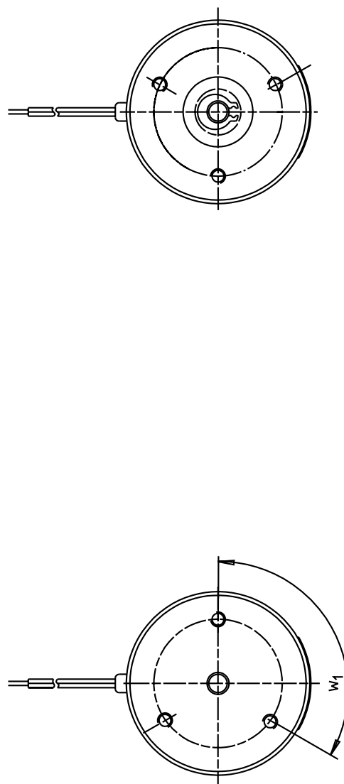
Fig. 15: hole pattern Type G DR X 075 X 20 A01
